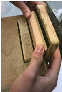
*Diagram showing placing the small piece of wood to make the lid snug but able to open*
