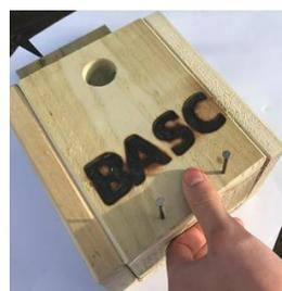
*Diagram front being attached using pre-drilled holes*
